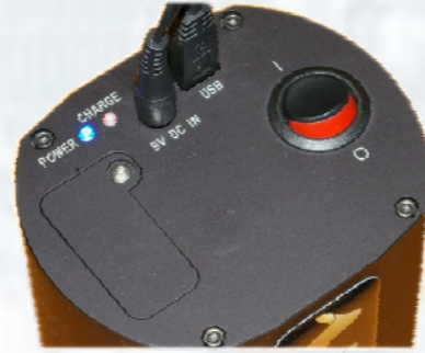
Internal Lithium Battery for handheld use – illumination with LED ring
